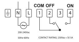
If mains voltage output is required, terminals L & 1 must be electrically linked. The cable link is provided with this timeswitch.
