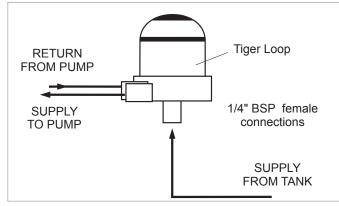
Figure 3-4: Tiger loop de-aeration device
