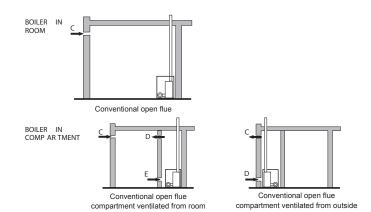
Figure 9-2: Air supply for conventional flue boilers
