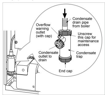
Figure 6-2: Condensate trap
