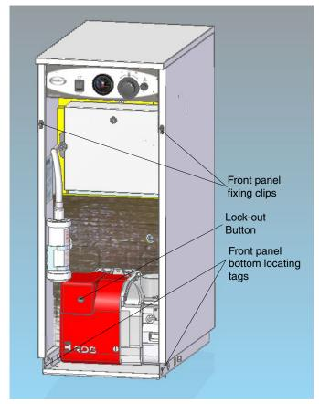
Figure 10-2: Position of boiler components - Vortex boiler
