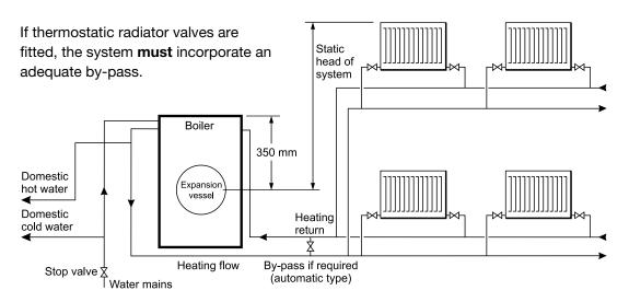
Figure 7-2: Sealed system boilers
