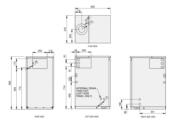
Figure 2-6: Vortex Utility 26/36, 36/46 and Utility System 26/36, 36/46 dimensions
