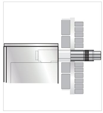
Figure 9-9: Low level balanced flue
