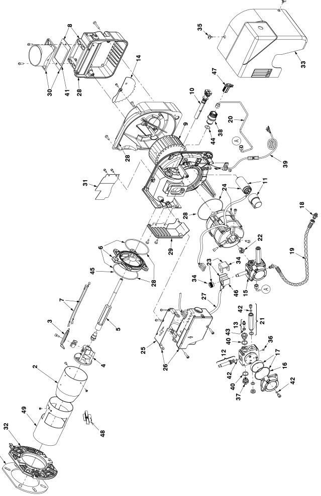
Figure 13-3: Riello RDB 2.2 BX burner exploded diagram - 15/21, 15/26, 26/36 and 36/46kW models
