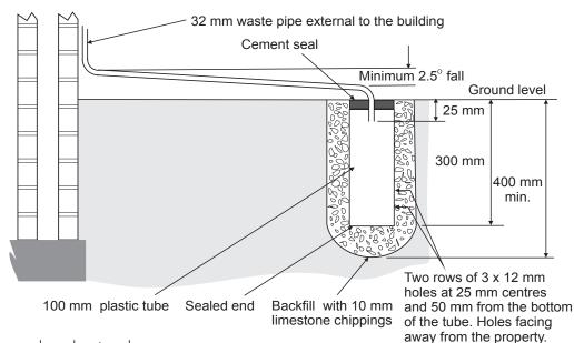
Figure 6-1: Purpose made condensate soakaway
