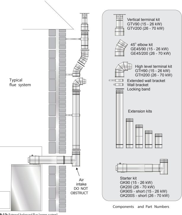
Figure 9-13: External balanced flue (green system)
