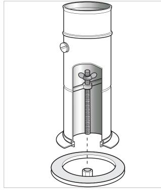
Figure 9-8: Boiler flue connector
