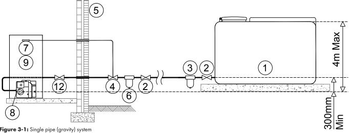
Figure 3-1: Single pipe (gravity) system
