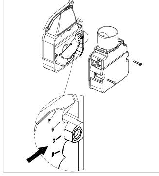
Figure 10-9: Air adjuster disc
