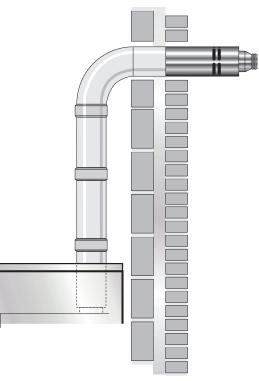
Figure 9-10: High level balanced flue
