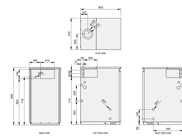
Figure 2-5: Vortex Utility 15/26 and Utility System 15/26 dimensions
