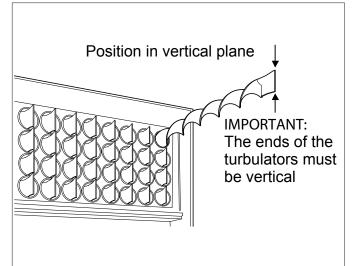
Figure 11-6: Turbulators Product codes: CA3261(INT-15-21KW) CA3360(INT15-26KW,26-36KW/36-46KW) CA3476 (INT-46-58KW/58-70KW).
