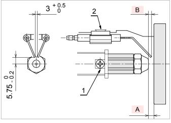
Figure 10-7: Ignition electrode settings
