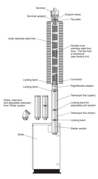
Figure 9-12: Red system balanced flue
