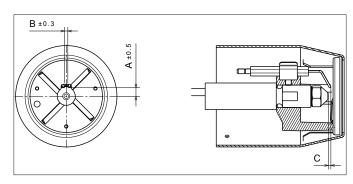
Figure 10-4: Ignition electrode settings
