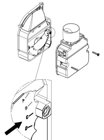
Figure 10-7: Air adjuster disc
