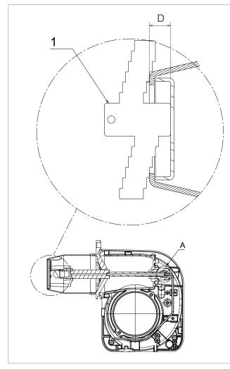
Figure 10-6: Diffuser position and gauge plate
