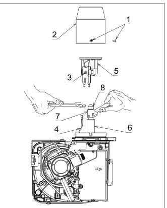
Figure 10-4: Burner head, diffuser and nozzle holder
