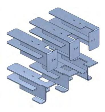
Figure 11-1: Baffles in Vortex Pro Combi 21
