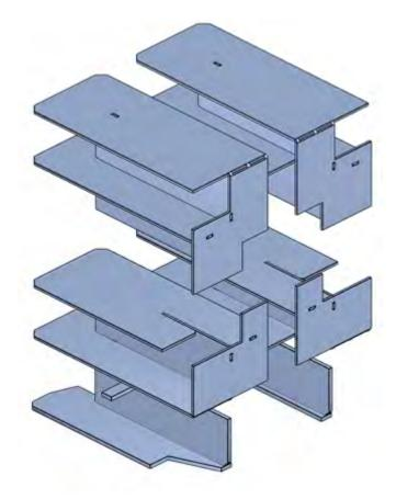
Figure 11-3: Baffles in Vortex Pro Combi 36
