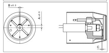
Figure 10-5: Ignition electrode settings
