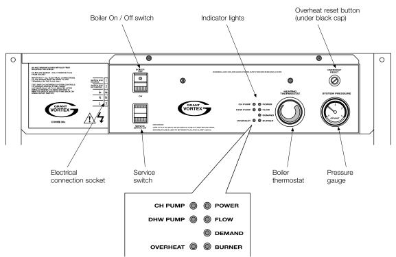
Figure 10-1: Vortex Pro Combi boiler control panel
