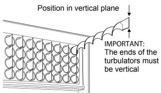
Figure 11-4: Turbulators in Vortex Pro Combi boilers
