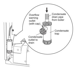
Fig. 15 - Condensate trap )Indoor/Utility models)
