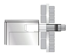
Fig. 17 - Low level balanced flue
