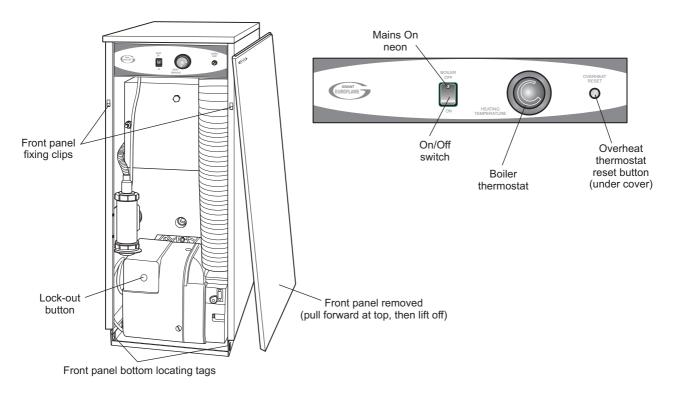
Fig. A Boiler controls (Indoor/Utility model shown)
