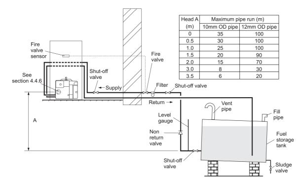
Fig. 4 - Two pipe system
