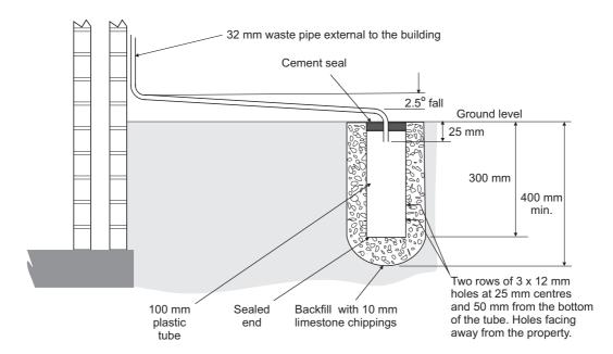
Fig. 14 - Purpose made condensate soakaway
