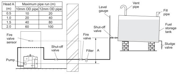
Fig. 3 - Single pipe system
