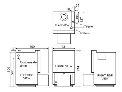
Fig. 1d - 90/120 Boiler House dimensions
