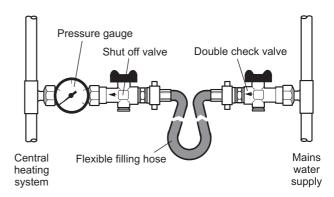
Sealed system filling loop arrangement - Fig. B
