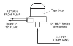
Fig. 6 - Tiger loop 'de-aeration' device
