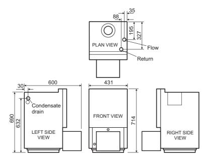
Fig. 1c - 50/70, 70/90 Boiler House dimensions
