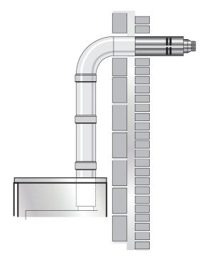
Fig. 18 - High level balanced flue
