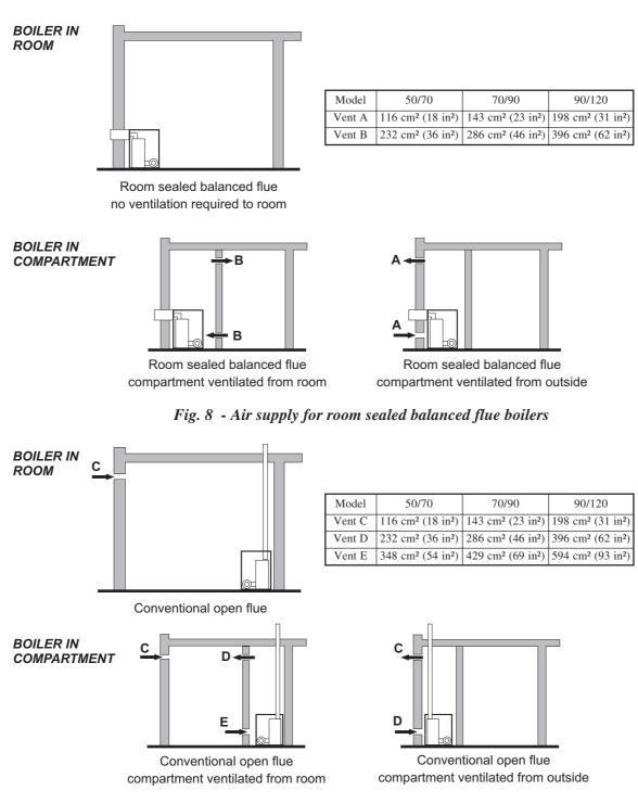
Fig. 9 - Air supply for conventional flue boilers
