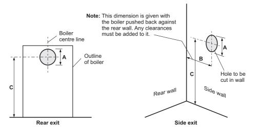
Fig. 17a - Low level balanced flue (Yellow System)
