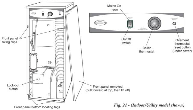
Refer to Fig. 21 for boiler controls
