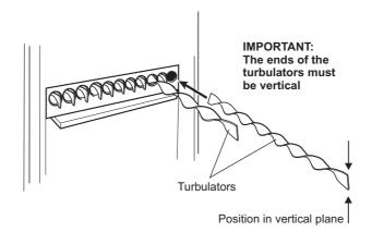
Fig. 25 - Turbulators (50/70, 70/90 shown)
