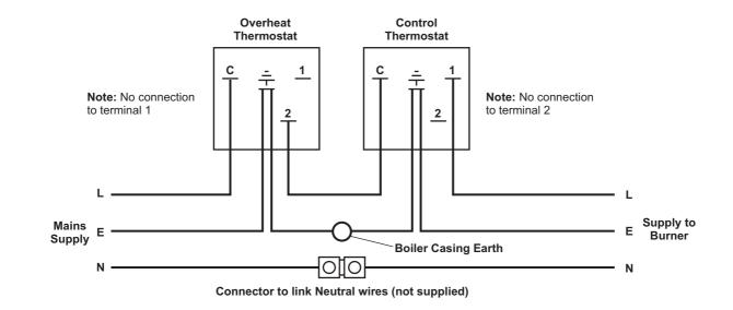
10.3 Dual thermostat wiring diagram - Boiler House models
