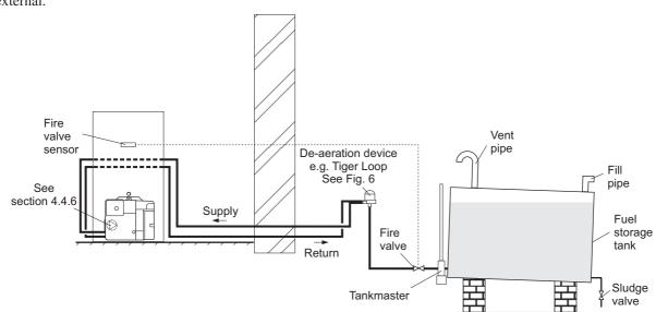
Fig. 5 - De-aeration device system
