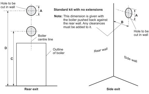
Fig. 18a - High level balanced flue (White system)
